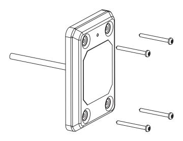
0. Make small recess or hole (diameter is 14 mm) to connect cable under the reader's case
