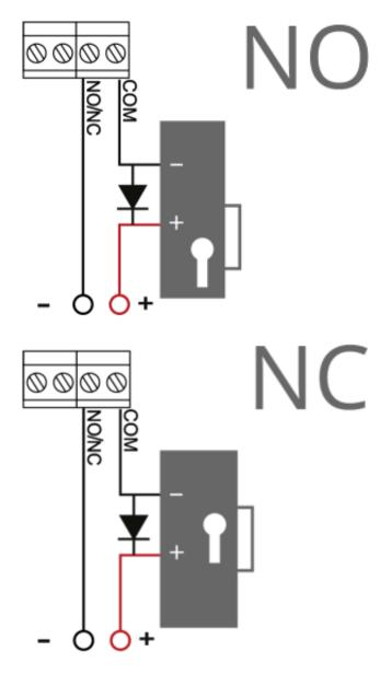
When using the relay contacts to control an inductive load (e.g., an electromagnetic lock), a flyback diode should be installed in reverse across the coil power supply to avoid contact damage.
