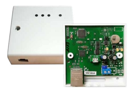
Intelligent controller for the organization of a global anti-pass back system (antipassback).
