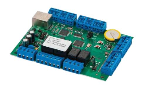
IP access controller that can work as part of the U-Prox WEB ACSon a wired computer network.
