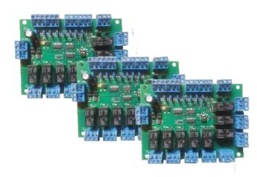
Controller is designed to organize an access control system on the floors of the building.
